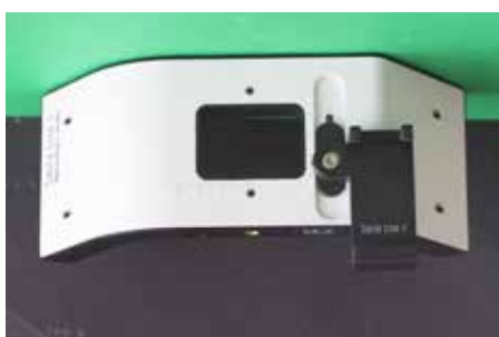
Figure 2. The Smile Line device showing the securing mechanism for the patient's mobile phone with its integrated camera.
