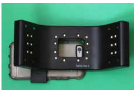
Figure 1. The Smile Line device holding a mobile phone showing the lighting system.
